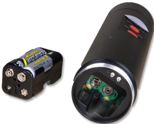
Figure 1B: ReferenceMate with battery holder removed from battery compartment
